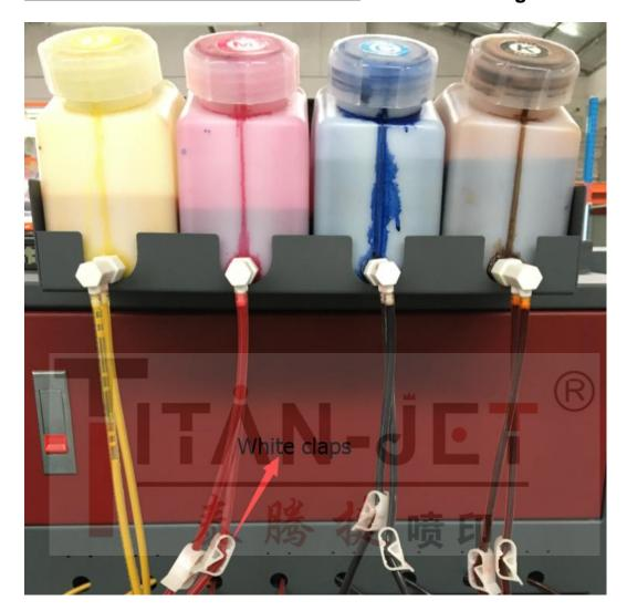
Warm Prompt: Must press this thin metal piece down enough to tighten the tubes, avoiding the tubes split away off. Otherwise it may burn the printhead or boards while the liquid drop out.
